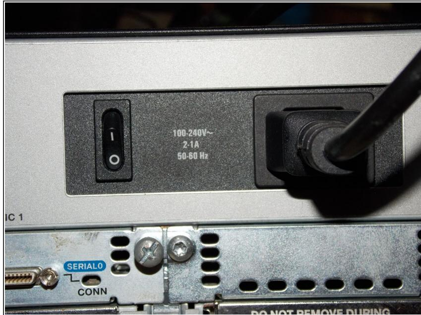
**⚠** In order to install or remove a card the equipment should be turned off.
