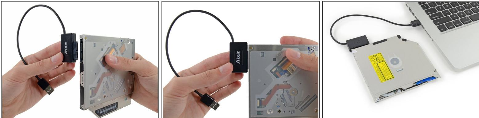
*(i)* Don't ditch that drive! You can still use your optical drive externally with the help of our [SATA Optical Drive USB Cable](#).
