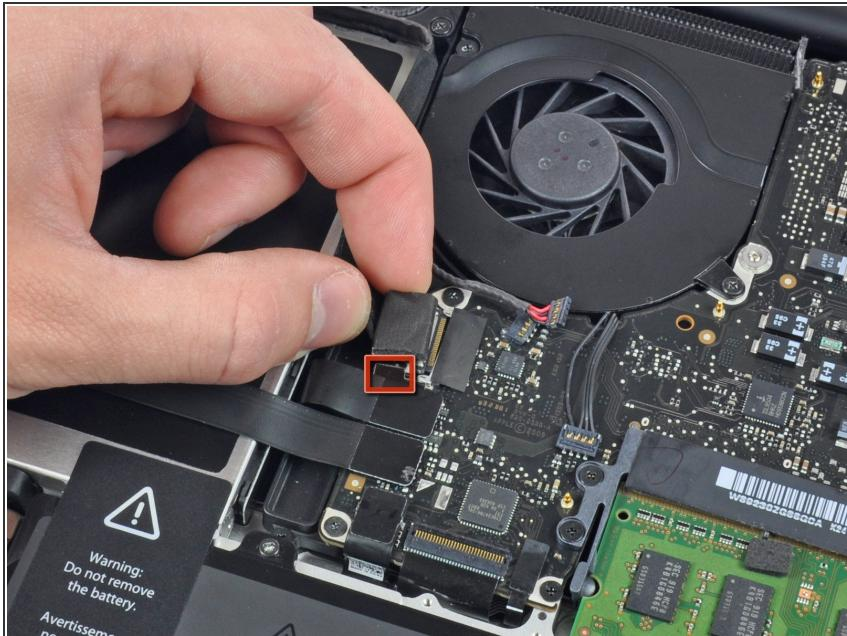
⚠ It will be necessary to slide the small clear plastic cable retainer (boxed in red) glued to the logic board out of the way before disconnecting the camera cable. Be careful not to break any components off the board as you slide it away from the camera cable connector.
