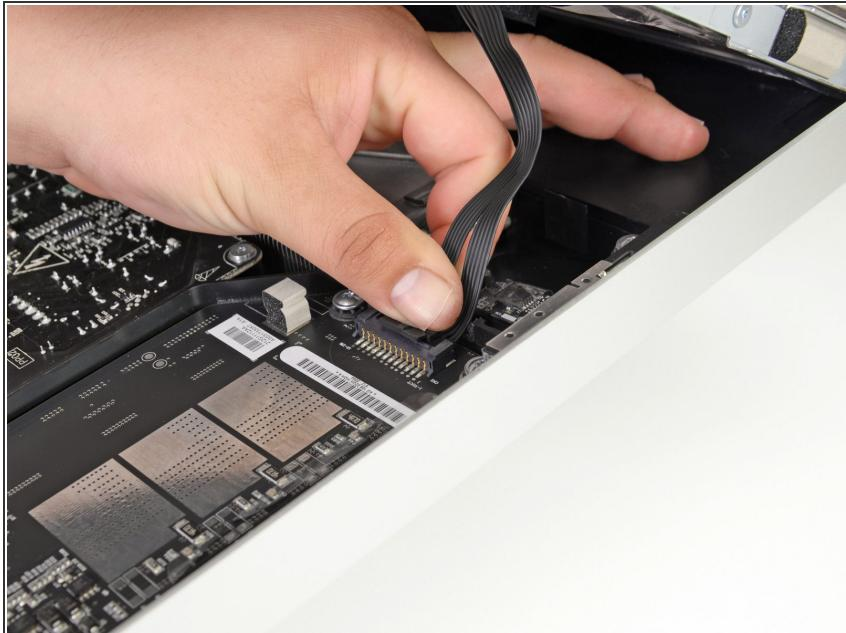
**⚠** This step brings your hands close to the exposed rear of the power supply. To avoid a high-voltage shock from the many large capacitors attached to the board, do **NOT** touch the rear of the power supply.
