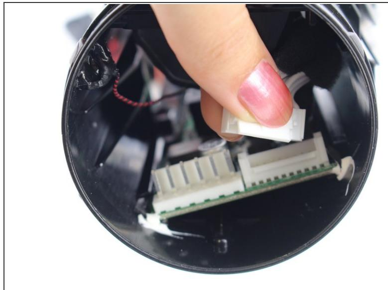
*(i)* Before removing port bay you must detach the connecting tabs on either side of the device.
