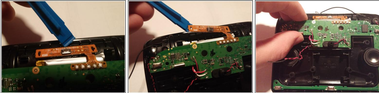
**⚠** Excessive force may cause the circuit board to break, destroying the device.
