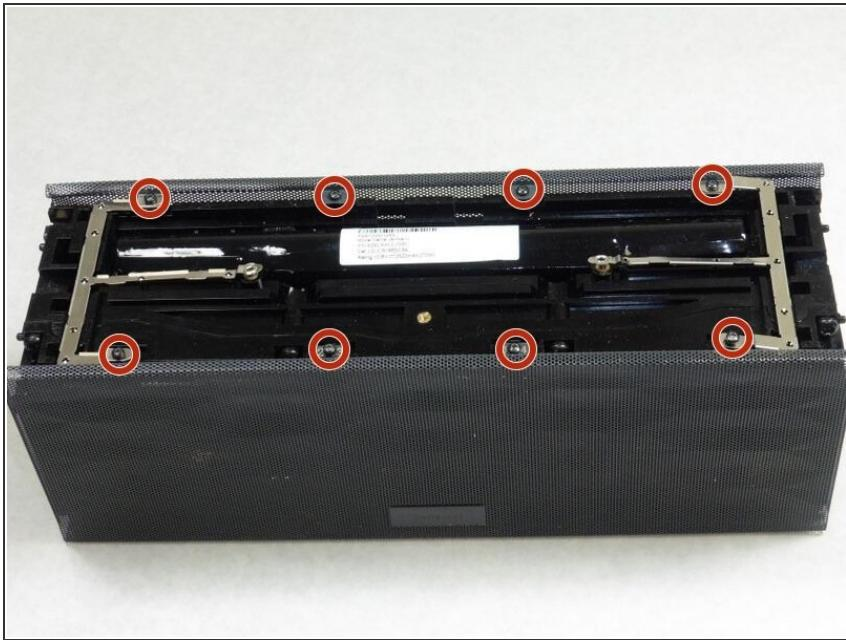
*(i)* Before unscrewing, take a picture of the top view. That way, when you're reassembling the device, you'll know the orientation of the metal grounding plates.
