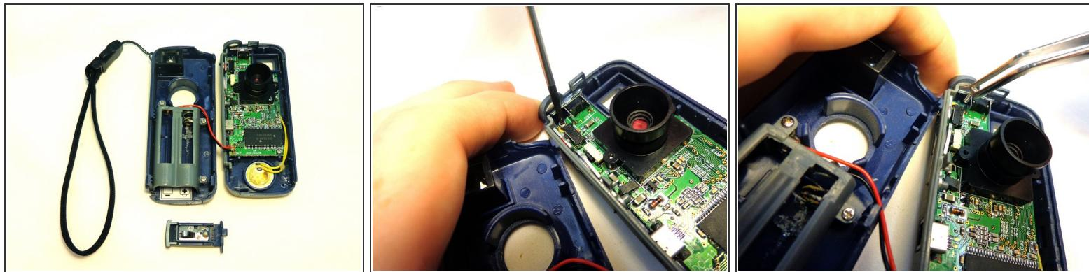
**⚠** There are two wires (one red and one black) that could get disconnected from the motherboard when prying the case apart.
