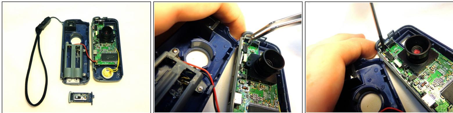
**⚠** Make sure to take care in prying case apart. There are two wires (one red and one black) that could get disconnected from the motherboard.
