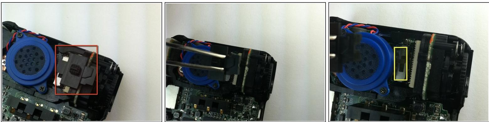
★ Before removing the switch, note its position for easy reassembly.
