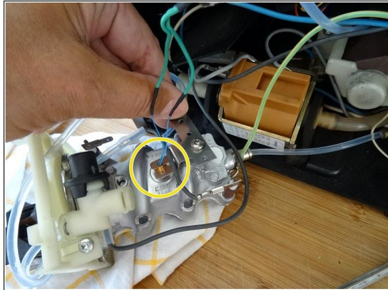
*(i)* The temperature sensor is fastened with a holding plate and a Torx 20 screw.
