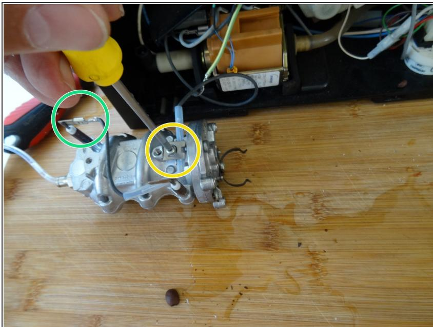
*(i)* There is a thermal fuse on the gray cable between the heater and the pump. It is attached to the heating cartridge with a retaining plate.
