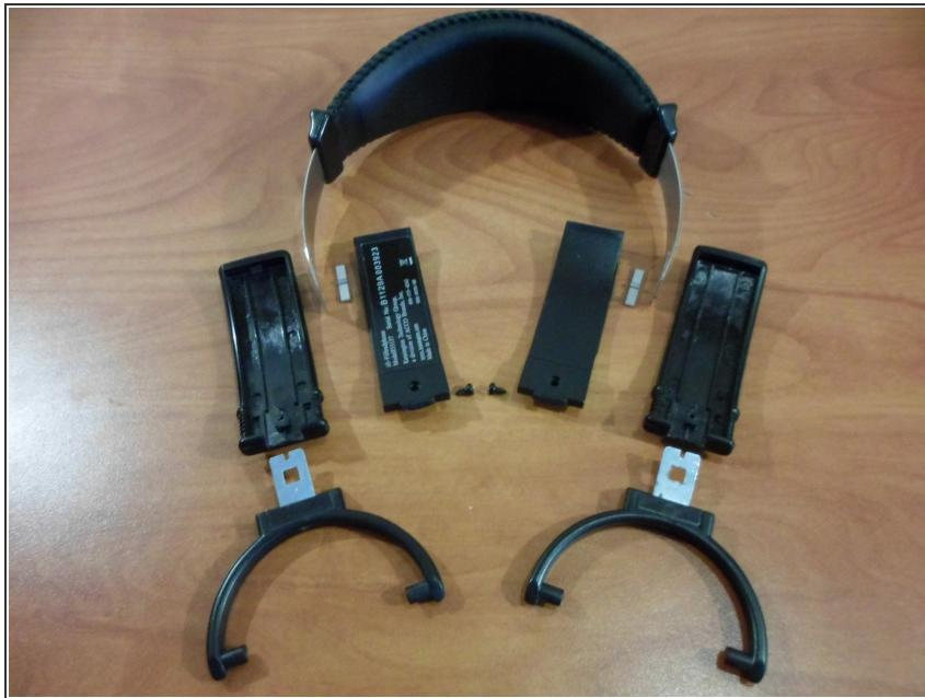
*(i)* All steps must be followed on both the left and right arms of the headband to free it completely from the outer coverings.
