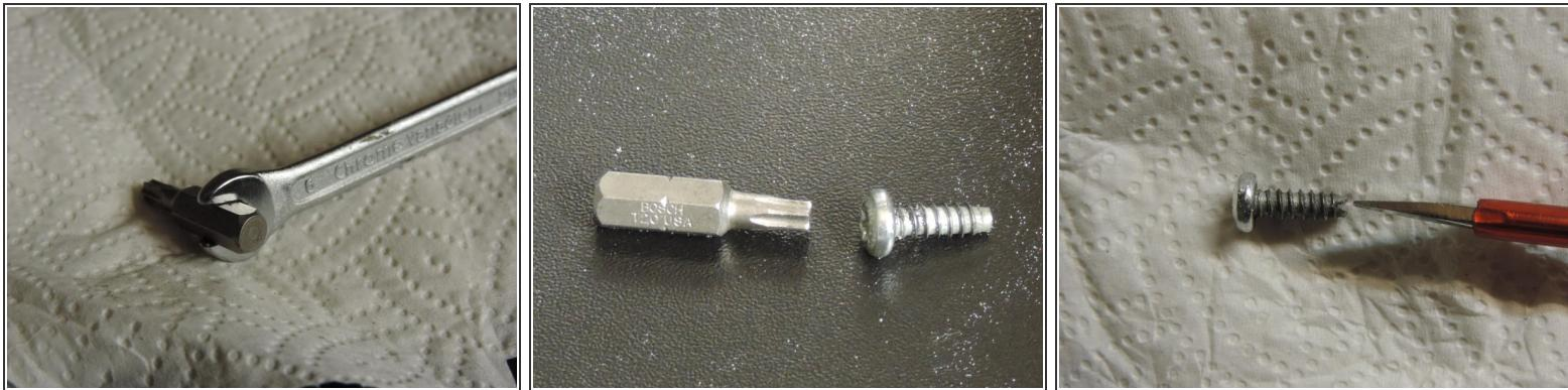
ⓘ I modified an open end wrench to drive a Tx20 bit
