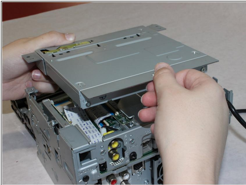
⚠ Lift the CD drive carefully to expose the attached cable underneath.
