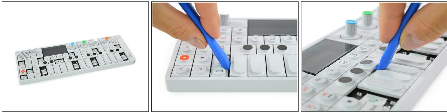
*(i)* To get to the screws beneath the keyboard you need to take some keys off. You can use either an opening tool or an opening pick. The first picture shows how it should look like with all the necessary keys off (12 in total).
