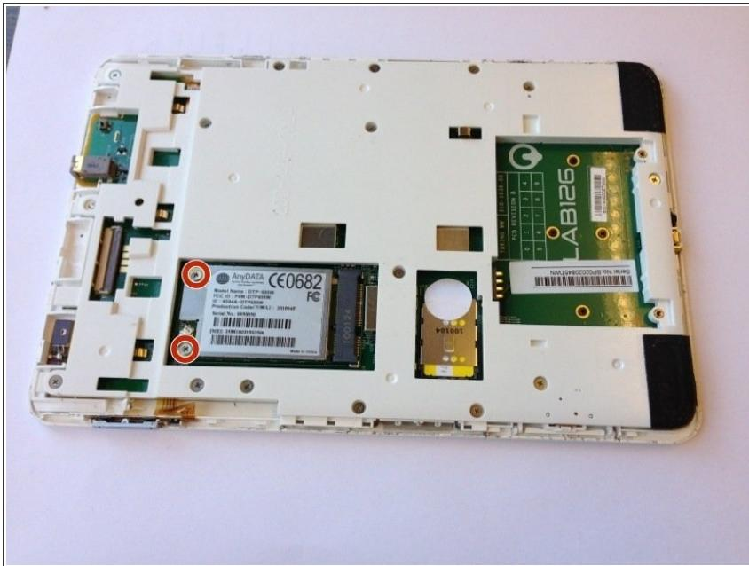
ⓘ Rotate the Kindle 180 degrees. Locate the wireless card with the AnyData logo on the top left and the FCC symbol on the right.
