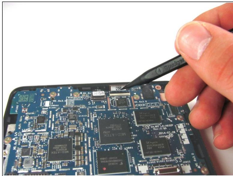
**⚠** Zero insertion force connectors can break easily. Before performing this step, read the [iFixit Guide to Recognizing and Disconnecting Cable Connectors](#) to find out how to safely remove them.
