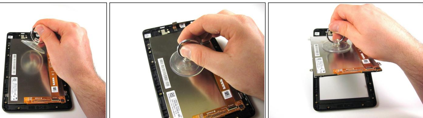
**⚠** Be careful not to scratch the screen while you're removing it. After you've removed the screen, place it on a cloth or another smooth surface to make sure that you don't scratch it once it is out of the device.
