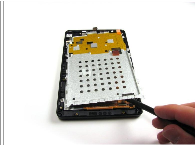
**⚠** An orange tape that connects to the motherboard runs through the metal plate. When removing the plate, be careful to maneuver the plate around the tape, and make sure not to stretch or rip the tape.
