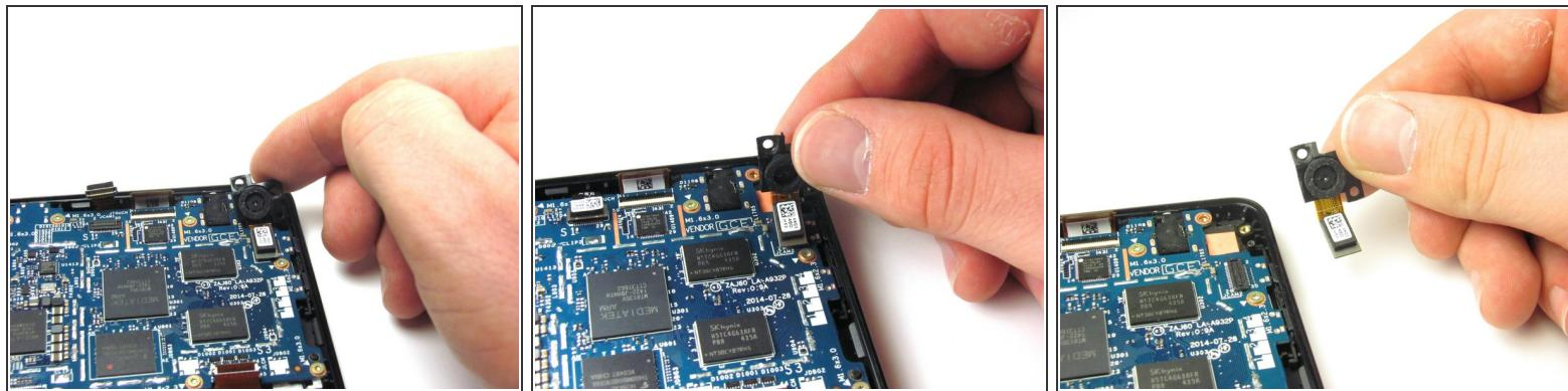
**⚠** Be careful not to damage the camera lens as you remove the camera.
