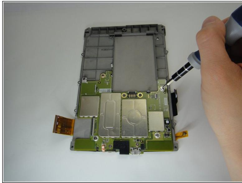
Use a Philips screwdriver to remove the seven 3.0 mm Phillips screws securing the motherboard:
