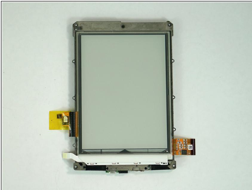
*(i)* The touchscreen is attached to the rest of the frame. Purchasing a new frame will require reattaching the motherboard and the battery.
