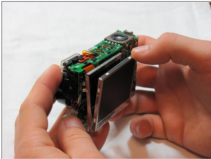
*i* The LCD screen is hinged at the bottom.
