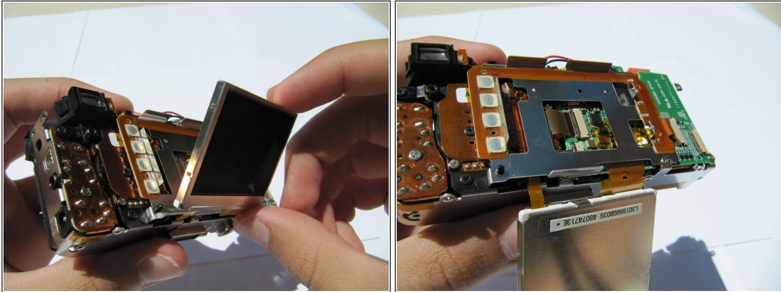
⚠ Carefully flip the LCD panel to expose the central circuit board.
