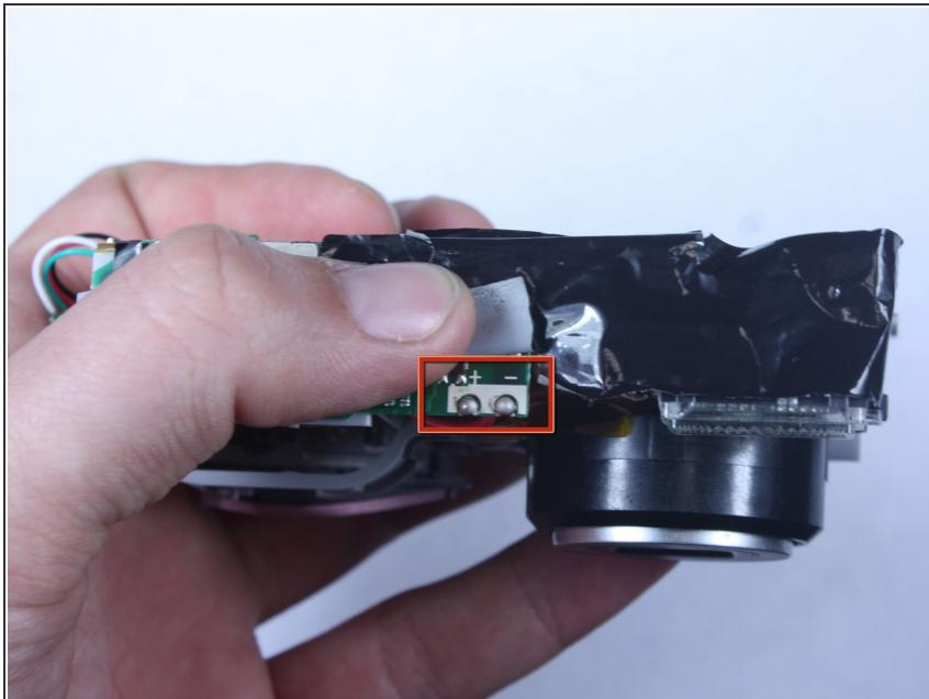
**⚠** Do not touch the terminals shown in the photo. These link to the capacitor which could shock you if not discharged.
