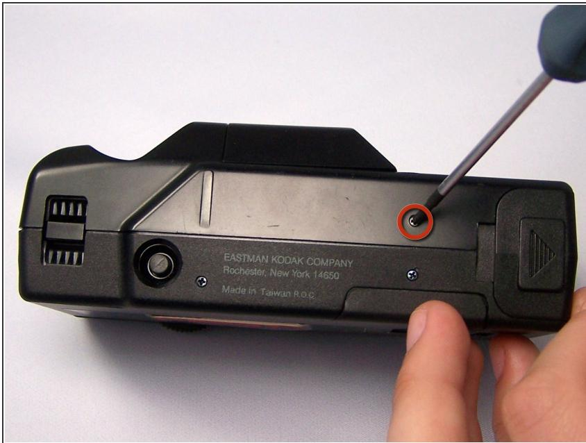
*(i)* Turn the camera so the bottom is facing up with the front facing away.
