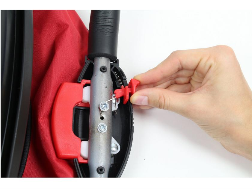
**⚠** The spring may pop out while removing the "Free Stand" button, so lift the button slowly to avoid losing the spring.
