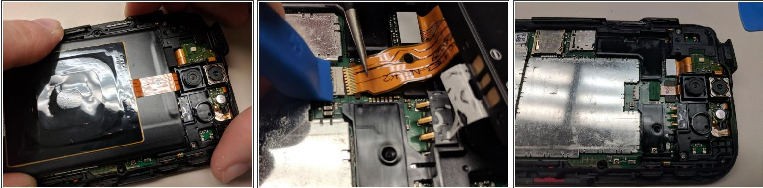
**⚠** Highly recommend making sure you are grounded before removing the battery. You will be handling areas that could cause damage if you accidentally create a static discharge.
