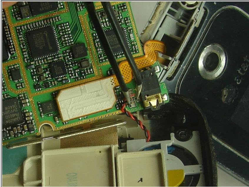
**i** Once the motherboard is not locked in place it will still be attached to the back phone casing by two wires, red and black, twisted together.
