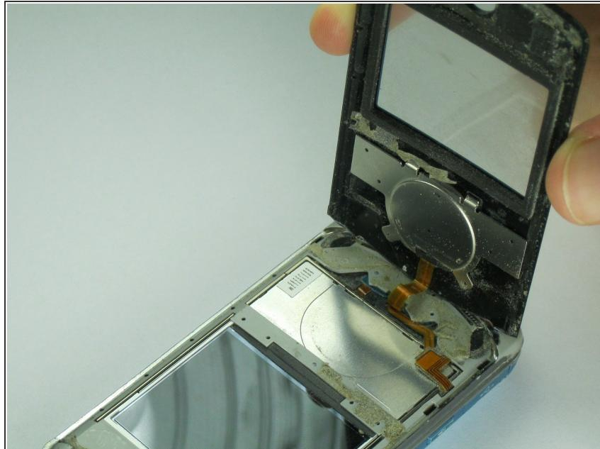
**!** The scroll wheel has an orange display data cable attached which may rip from excessive force.
