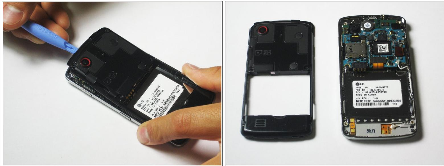
**⚠** In the next step, be gentle with the plastic back case when prying it away from the phone because it is attached with adhesives on the bottom side of the phone. If you try to force the back case off, you may crack it.
