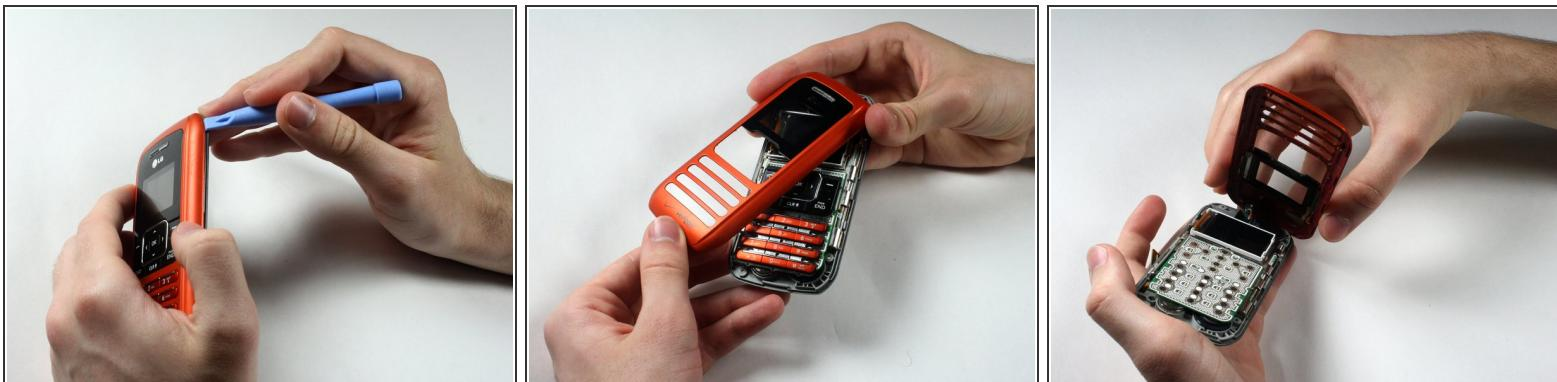
! Be careful while breaking the adhesive connecting the speaker and the casing in the following sub step so that you do not tear any wires.
