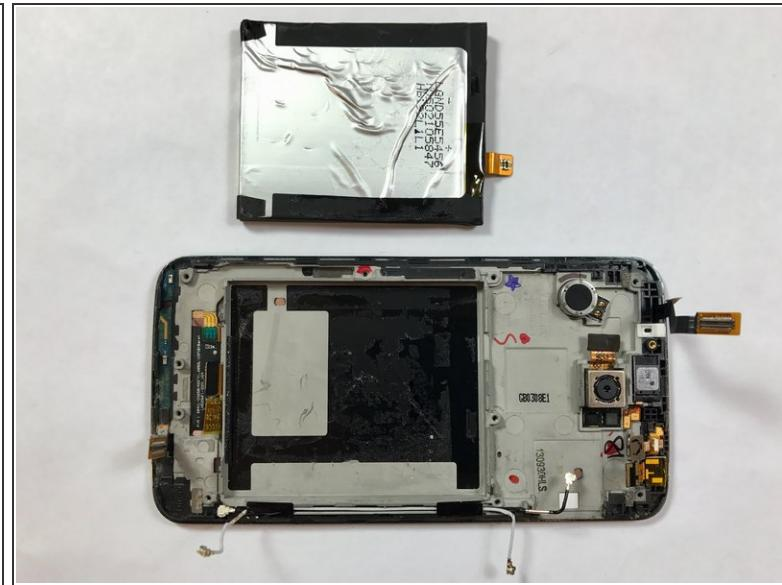
**⚠** Now you are ready to remove the battery. Make sure to adhere to ESD prevention guidelines, use a plastic tool as to not damage the battery.
