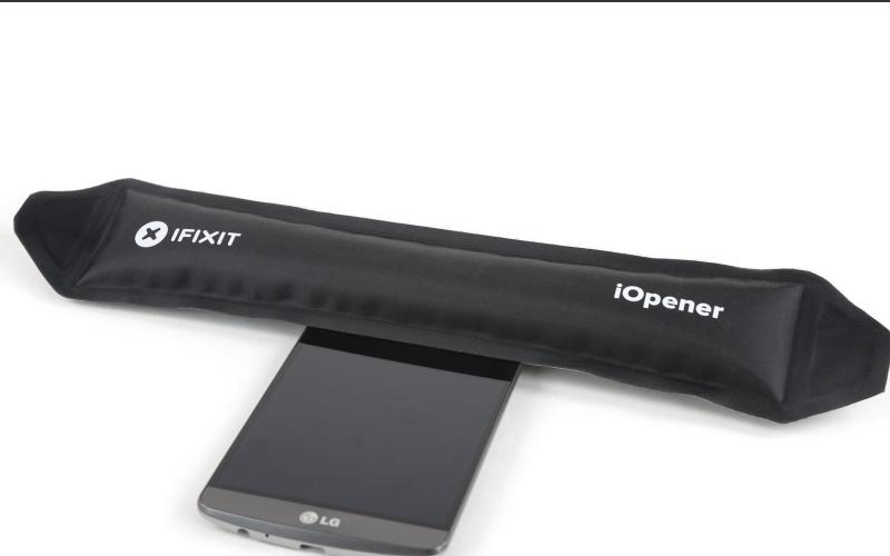
*(i)* [Apply a heated iOpener](#) to the top end of the screen to loosen the adhesive underneath.
