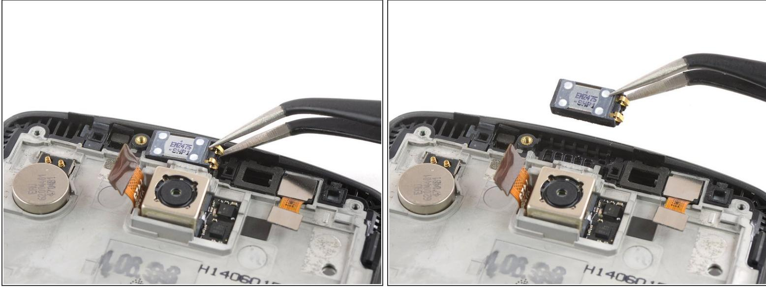
⚠ During the removal of the earpiece speaker, remove it together with the foam gasket underneath.
