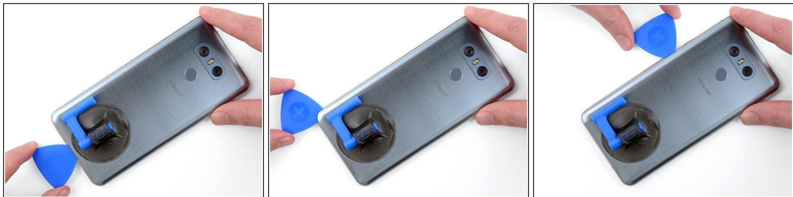
ⓘ As you proceed with separating the adhesive, you might need to re-apply heat to each edge before you can slice the adhesive securing it.
