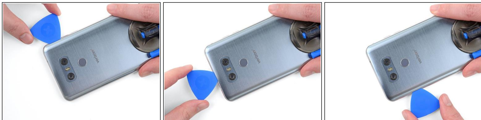
! As seen in [Step 1](#), the fingerprint reader cable runs to the left of the camera, fairly close to the edge of the phone. Be careful as you cut through the adhesive in the upper edges of the phone.
