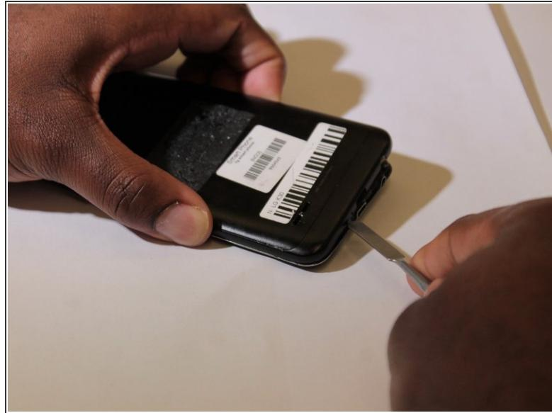
**⚠** Before disassembling your LG K30, discharge the battery below 25%. A charged lithium-ion battery can catch fire and/or explode if accidentally punctured.
