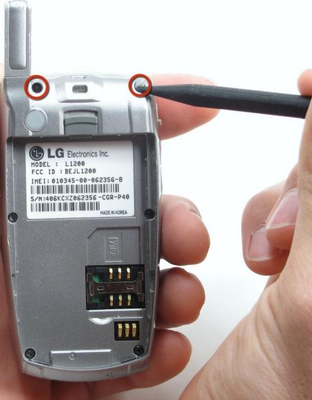
**⚠** Make sure you remove the battery by lifting the tab on the back of the phone before opening the case.
