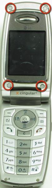
⚠ Make sure you remove the battery by lifting the tab on the back of the phone before opening the case.
