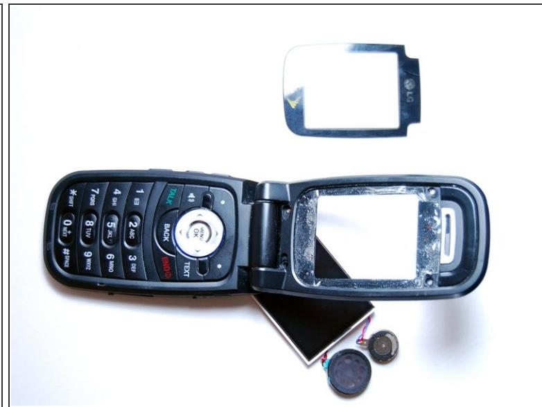
⚠ Apply even amounts of force upon removing screen, otherwise cracking may occur.
