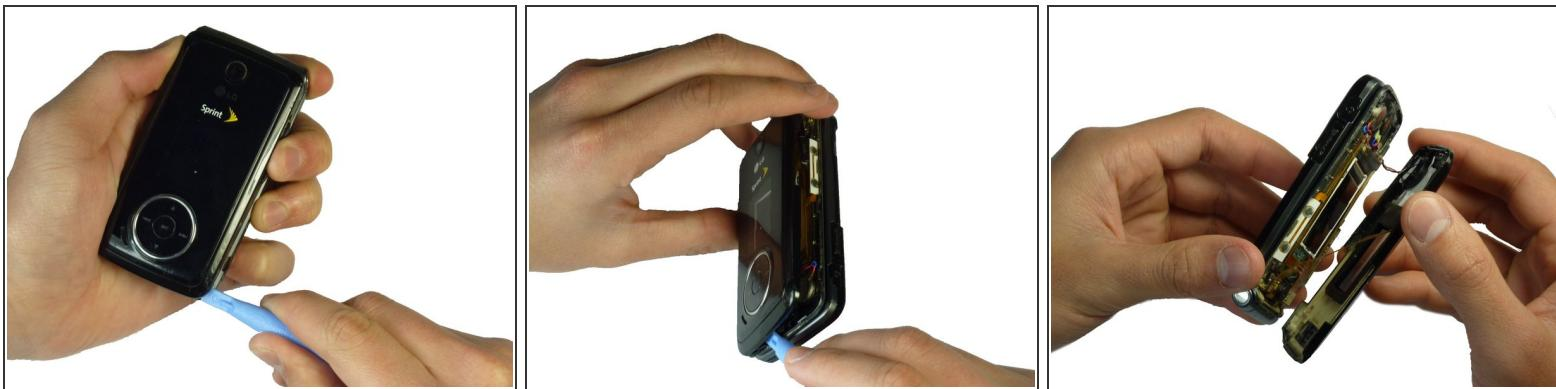
**⚠ Caution:** Wires and ribbon connect the front case to the main body. Exhibit care when separating front case from the main body as to not break the connections.
