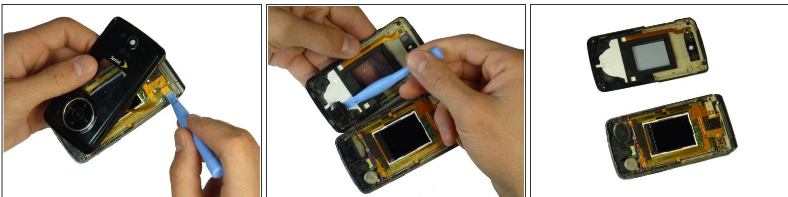
**⚠ Caution:** The wires and ribbon connector can break easily. Exhibit care when removing them.
