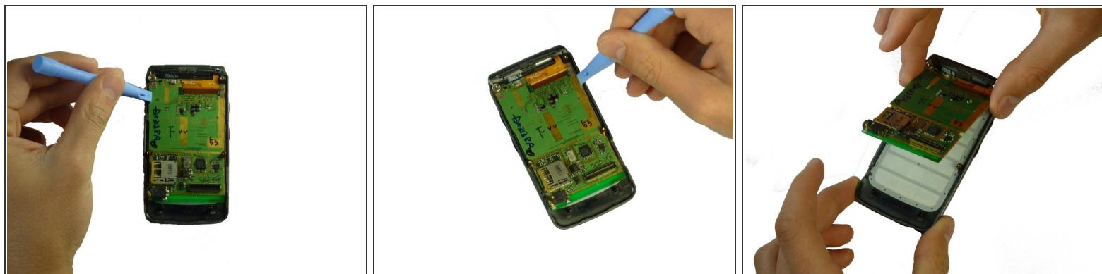
! **Caution:** The circuit board is connected via ribbon to the phone. Do not break this connection.
