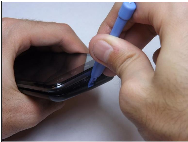
⚠ Make sure not to push the tool into the USB port. Doing so may cause damage to your phone.
