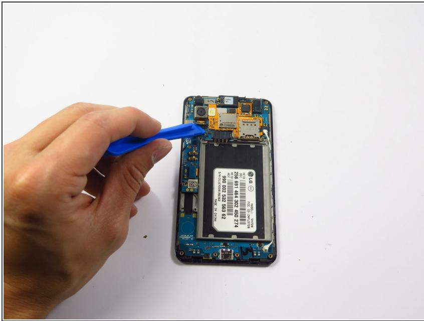
**i** The camera unit is located at the top left of the phone. The camera is a silver box with a black lens. The image pin points where the camera is on the motherboard.
