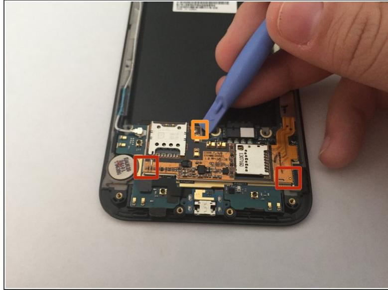
**⚠** In this next step it is easy to pry the wrong piece. Make sure to pry at the metal platform that the sister board sits on, not the orange printed circuit board itself.
