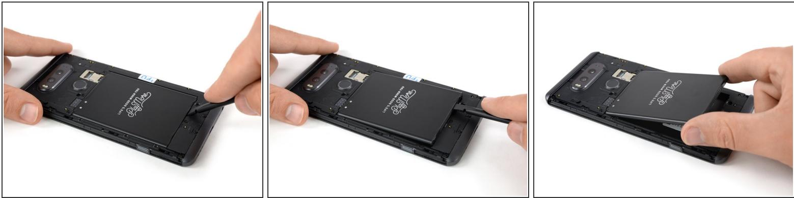
**⚠** Before disassembling your phone, discharge the battery below 25%. A charged lithium-ion battery can catch fire and/or explode if accidentally punctured.
