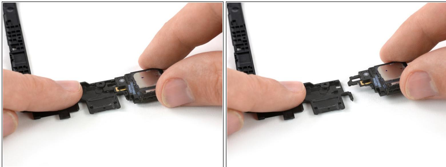
*(i)* The loudspeaker is attached to the cover of the motherboard by a tight plastic clamp.
