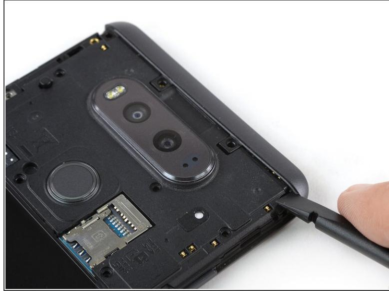
*(i)* The top and bottom frame section hold very tight to the mid frame. It is possible to pull them off with your hands. If you're not able to do so, use the following removal procedure:
