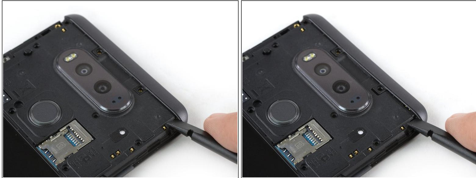
*(i)* The top and bottom frame section hold very tight to the mid frame. It is possible to pull them off with your hands. If you're not able to do so, use the following removal procedure:
