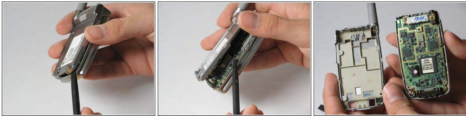
**⚠** Be careful when removing the casing as the spudger can damage the plastic cover of the phone.
