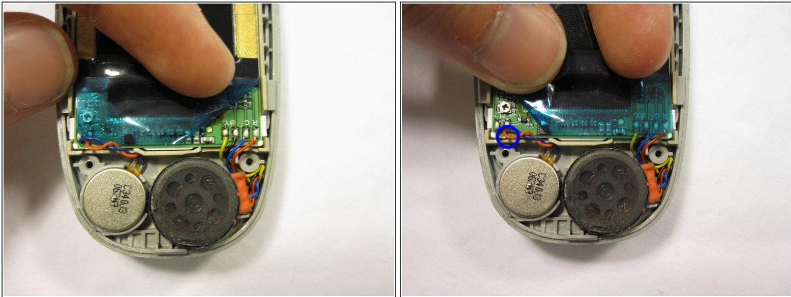
⚠ Try not to move the thin component wires as they will bend and break very easily.
