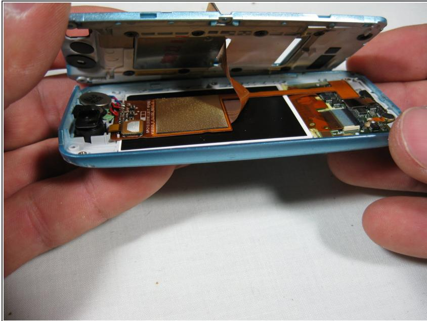
⚠ Carefully lift the slider mechanism to see the ribbon cables underneath.
