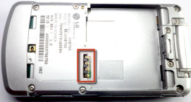
**⚠️** When installing the battery, make sure to align the metal pins with those of the phone.
