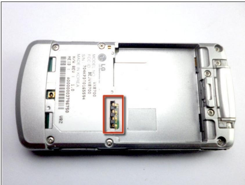
⚠ When installing the battery, make sure to align the metal pins with those of the phone.
